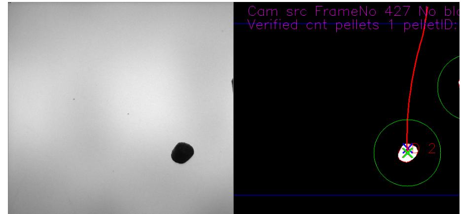
Figure 21 Pellet detection using image analysis. Raw image (left) and analyzed image (right).
