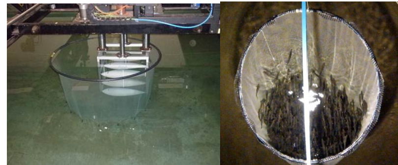
Figure 28 Left: Model tests with 9 rigid fish models in a fish cage. Right: Bird-eye view of model tests of a fish cage with 800 small salmon in current velocity 0.16 m/s.
