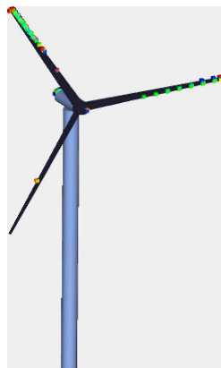
Lightning attachment points for the highest 2000 strikes <math><100\text{kA}</math>
