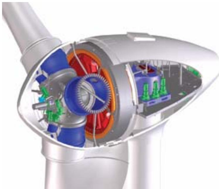
Figure 3: Schematic of Enercon 2 MW wind turbine. Copy from www.enercon.de .
