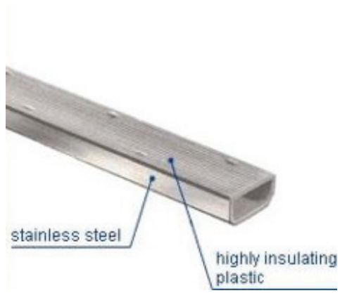
Figure 36. Thermix TX.N spacer. From http://www.fenestration-uk.com/News/NewsItemRSS.aspx?id=1885 .
