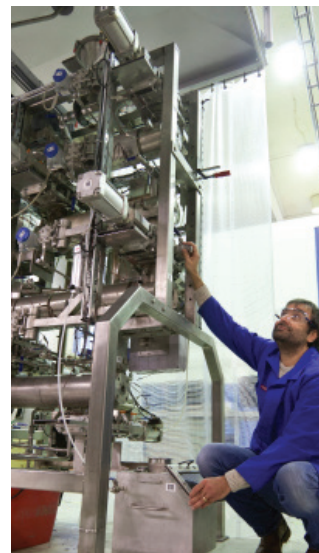
Torrefaction Reactor - a thermal pre-treatment process that enhances the properties of biomass.
