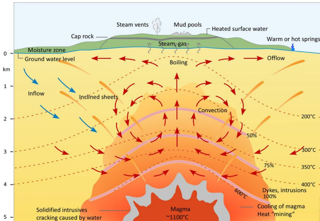
**Fig 1.** Geothermal field; conceptual model from Sæmundsson and Jónsdóttir (2010).
