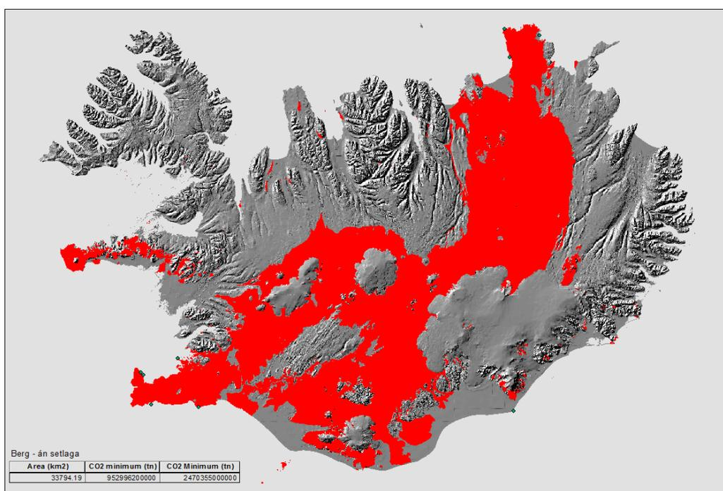
**Fig 3.** Theoretical area feasible for CO<sub>2</sub> mineral storage in Iceland; Basaltic formations from Holocene and upper Pleistocene, younger than 0.8 M yr.
