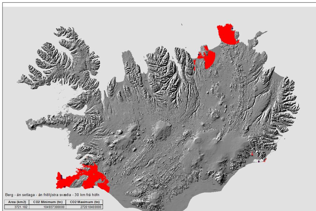
Fig 4. Theoretical area feasible for CO<sub>2</sub> mineral storage in Iceland; Basaltic formations from Holocene and upper Pleistocene in the vicinity (radius of 30 km) of a large-scale harbor.
