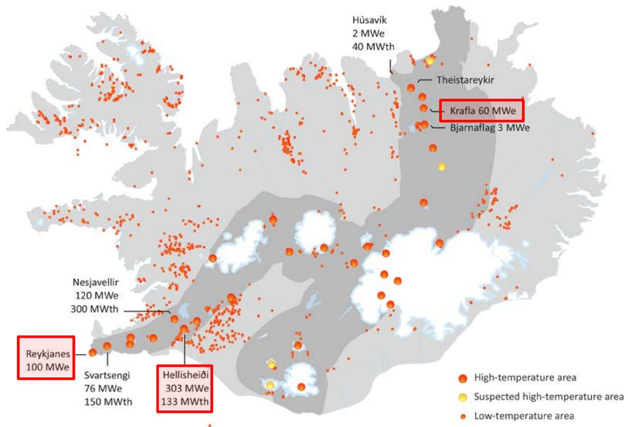
**Fig. 2** Geothermal map of Iceland (ÍSOR, 2013). High-temperature geothermal areas of concern in Wiese's study are marked with a red box as well as the present energy harnessed from the field in megawatts electricity production (MWe) and megawatts thermal water production (MWth).
