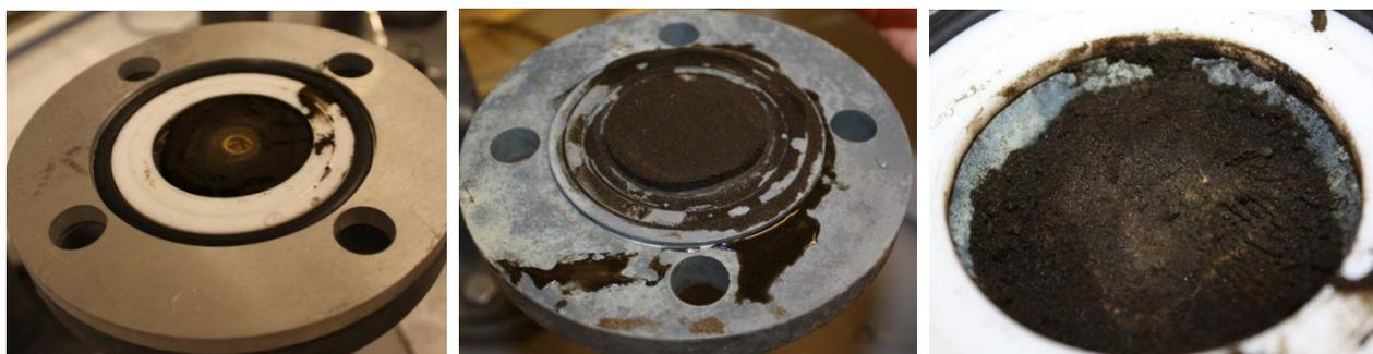
Figure 3. The appearance of the basaltic material glass in the first compartment after unscrewing the column reactor.
