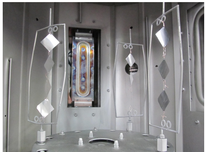
Linear Ion Source cleaning of substrates.
