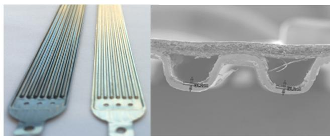
PVD coated and uncoated small scale BPPs (left), and combined GDL/BPP concept on stamped small size BPPs, where the GDL can be glued to the BPP with a non-conductive glue (right). SEM images for TiN-PANI coating with different coating time (below).
