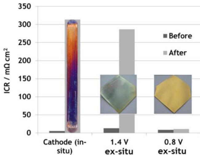
Comparing in-situ and ex-situ results, adjusting ex-situ test parameters (applied potential in ex-situ test 0.8 and 1.4 V for one hour).
