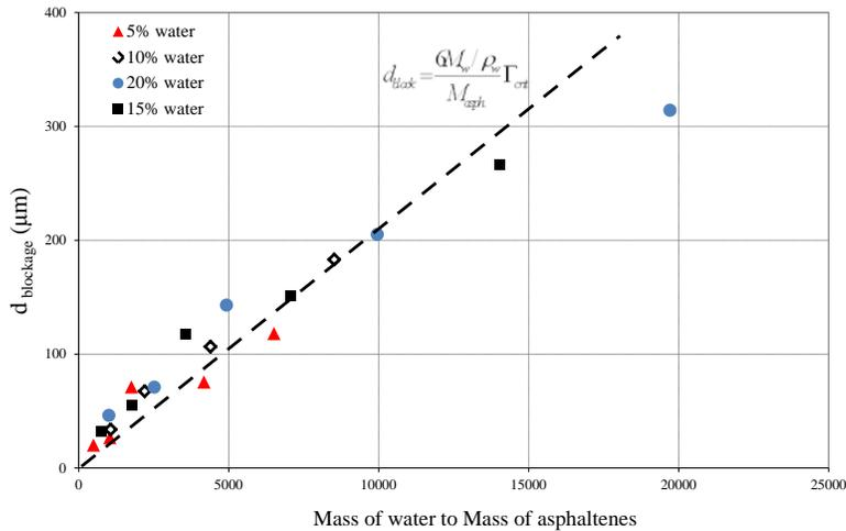
**Figure 3: Dependency of blockage diameter over mass of water/mass of asphaltenes.**
