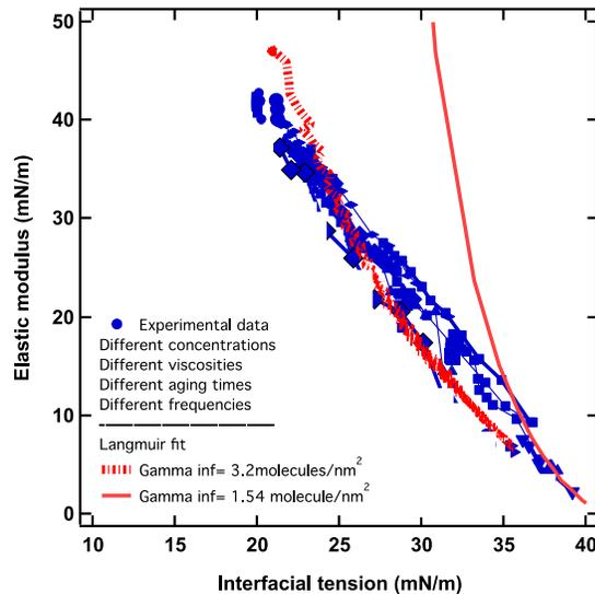
*Figure 2: Parametric curve instantaneous elasticity vs. interfacial tension from Langmuir equation of state (previously identified  $\Gamma_{\infty}=3.2$  molecules/nm<sup>2</sup> and arbitrary  $\Gamma_{\infty}=1.54$  molecules/nm<sup>2</sup> to show sensitivity) and comparison with experimental results.*
