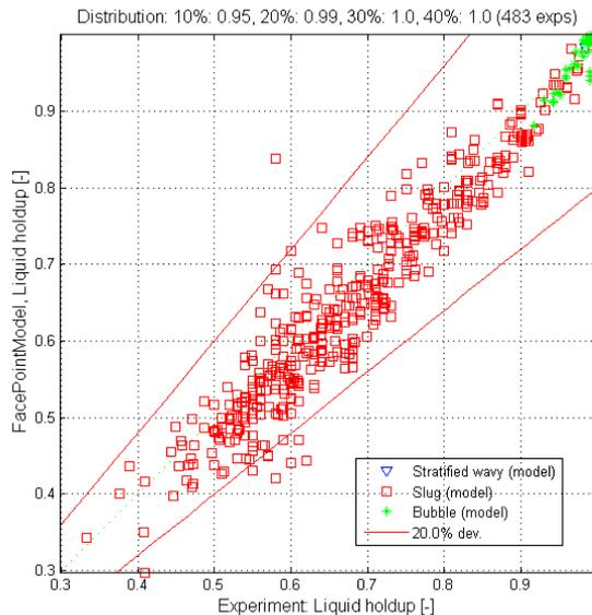
**Figure 6.** The figure shows the correlation between holdup in slug flow for the point model developed in FACE and several data sets available in the literature [Copyright by Jan Nossen, IFE].
