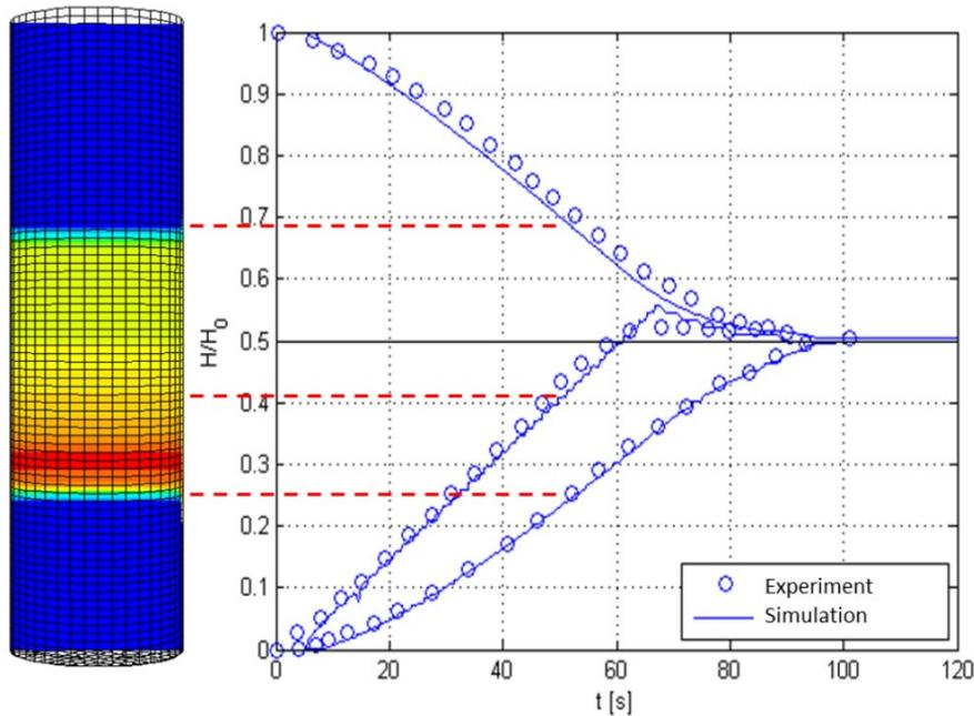
*Figure 4: Validation of DPL simulations in Fluent against experimental data.*
