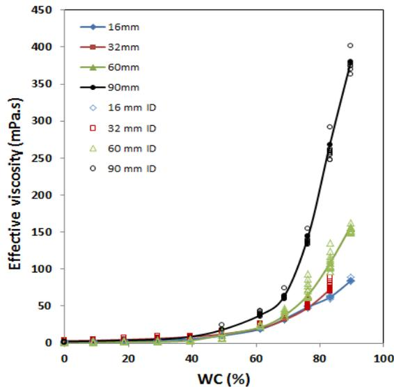
Figure 5 Effective viscosity as a function of pipe diameter [Copyright by Jose Plasencia, NTNU].
