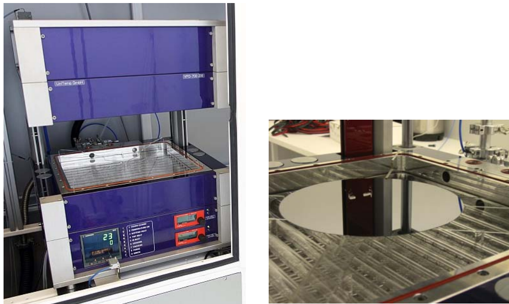
Figure 6: (left) RTP furnace opened; lower lamp array can be seen. (right) quartz carrier with 200 mm wafer; the carrier can also hold the sacrificial plate (not mounted)
