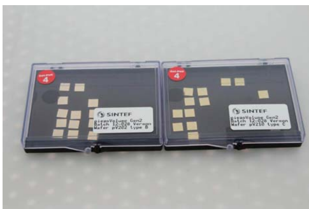
Figure 4-2: Generation 2 devices as delivered in Gel-Paks to Vermon. Left: 13 devices from process type B, Right: 12 devices from process type C (only 9 delivered)
