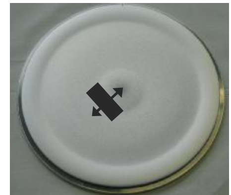
Movable position of inner magnets
