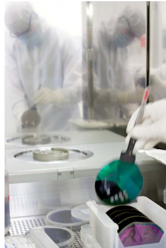
Release etch of piezoMEMS wafers
