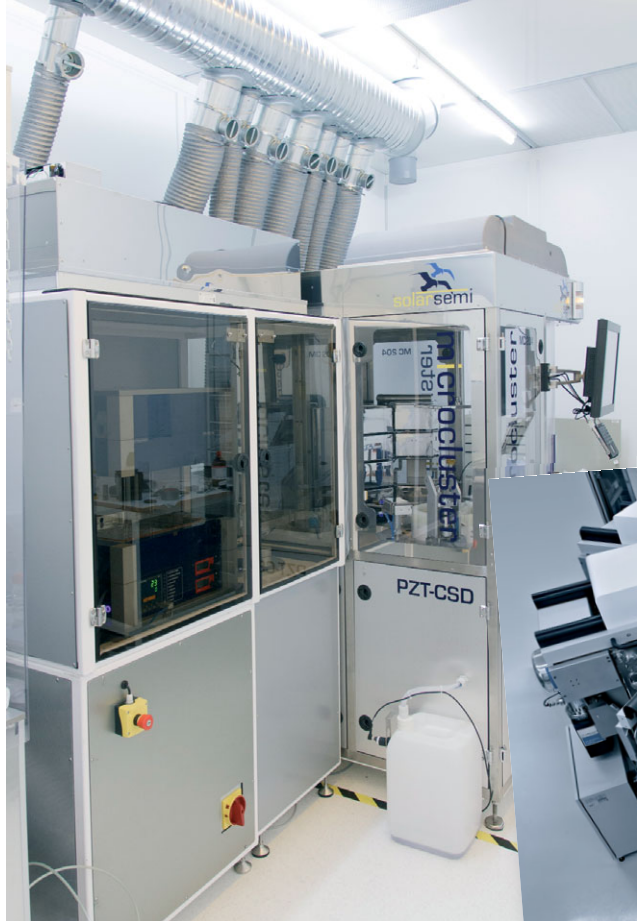
<< LEFT | Figure 2: PZT CSD cluster coating tool by Solar-semi. >>
