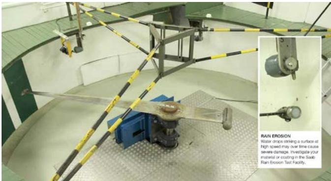
SAAB Rain erosion test facility
