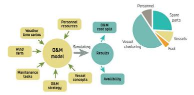
Schematic of inputs and outputs for the NOWIcob model
