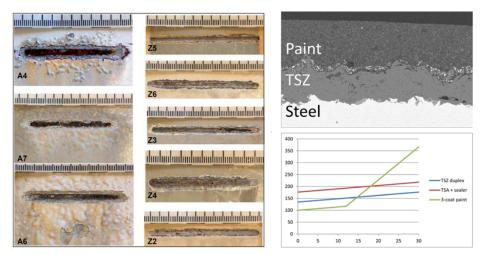
Pictures of some of the costing systems after exposure for five years in corrosive marine atmosphere. **A:** Coating systems with thermally sprayed Aluminium.
