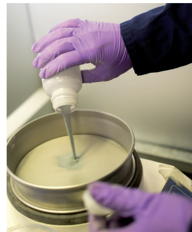
Figure 1: No one has ever been able to process silicon carbide in such a way that it can be sprayed as a coating on machine parts. That was before NOWITECH PhD student Fahmi Mubarak began his doctoral research. Read more about this work in chapter 8.5. Photo: synlig.no
