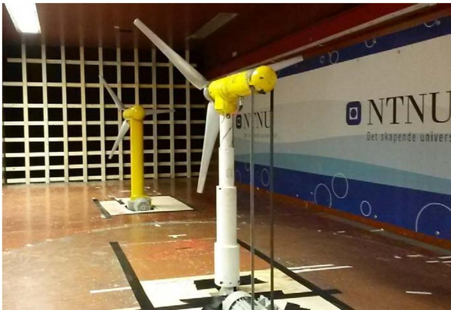
**Figure 7:** Turbine models exposed to highly turbulent shear flow
