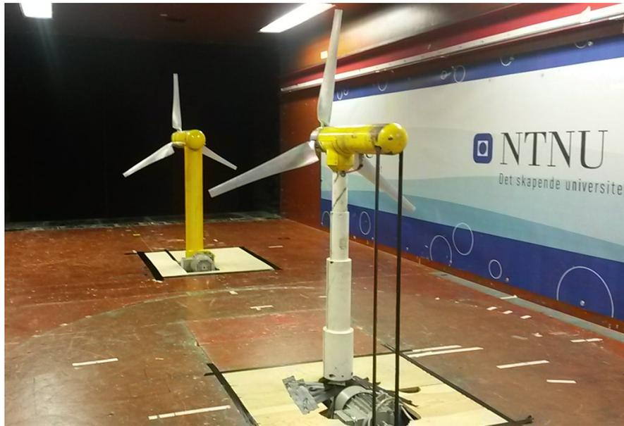
*Figure 5: Turbine models exposed to low turbulence inflow*
