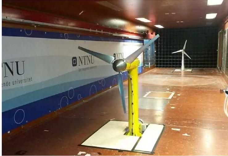
*Figure 1: Model wind turbines in the wind tunnel ( $x/D=9.00$ )*
