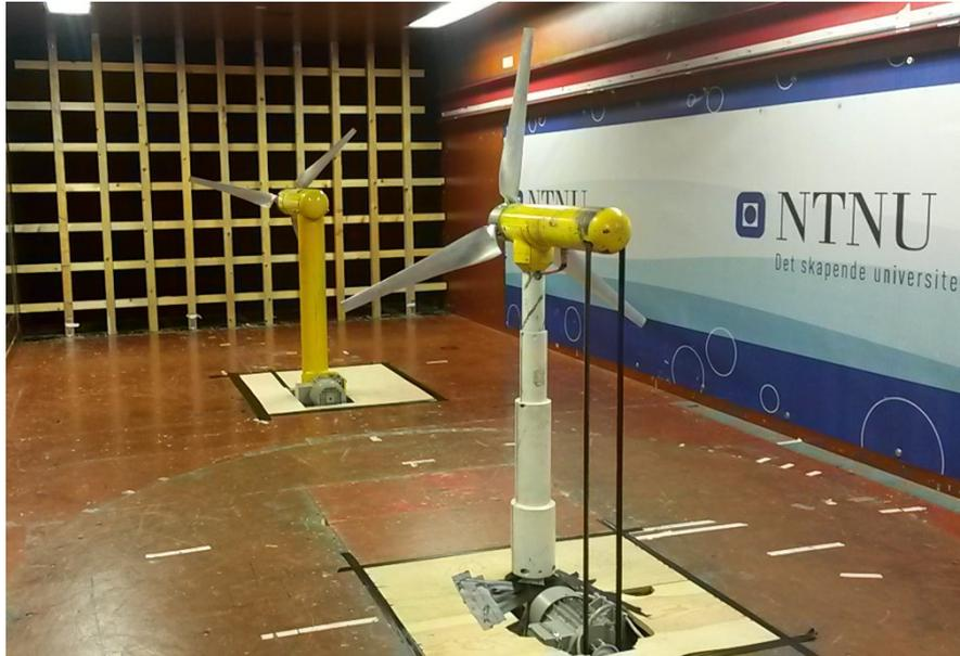
**Figure 6:** Turbine models exposed to high turbulence inflow generated by an evenly spaced grid
