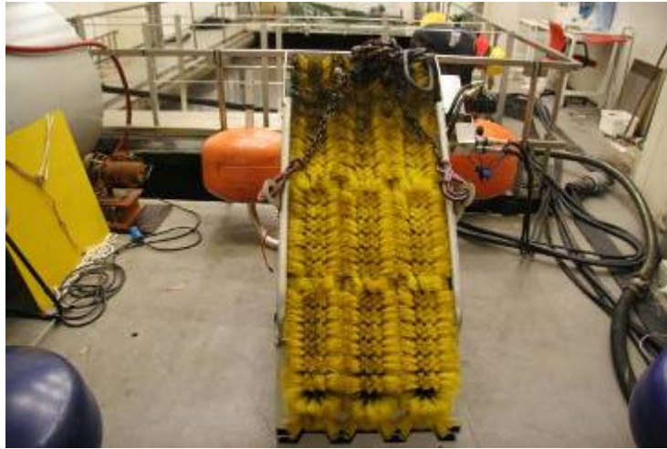
Figure 4.1 GT 185 Skimmer with brush conveyor, viewed from front
