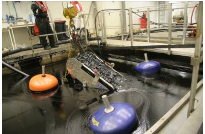
Figure 5.5 Flow of emulsion to the skimmer
