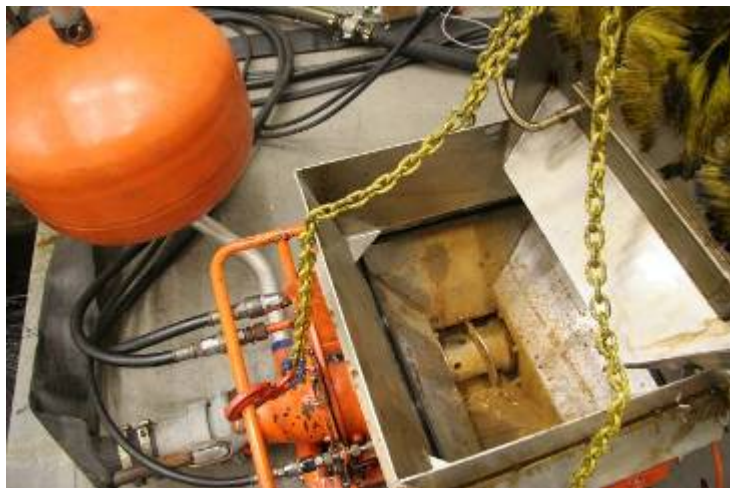
Figure 4.2 Sump for recovered oil and pump on the GT 185 Skimmer
