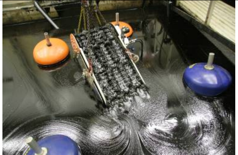
Figure 5.4 Flow of emulsion to the brush conveyor
