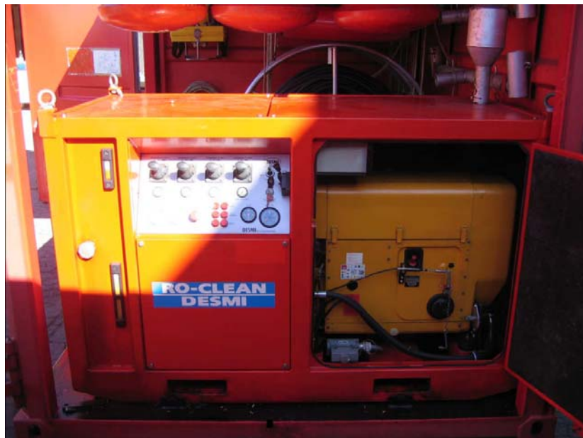
Figure 4.5 Diesel hydraulic power pack used during the tests.
