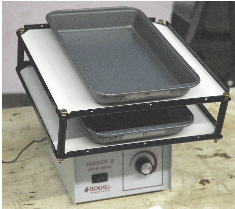
Figure 1: Rocking shaker with two platforms for experiments with a DFP test tray on each platform.
