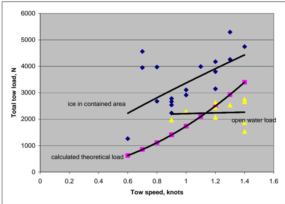
**Figure 6: Tow loads on AFTI boom**
