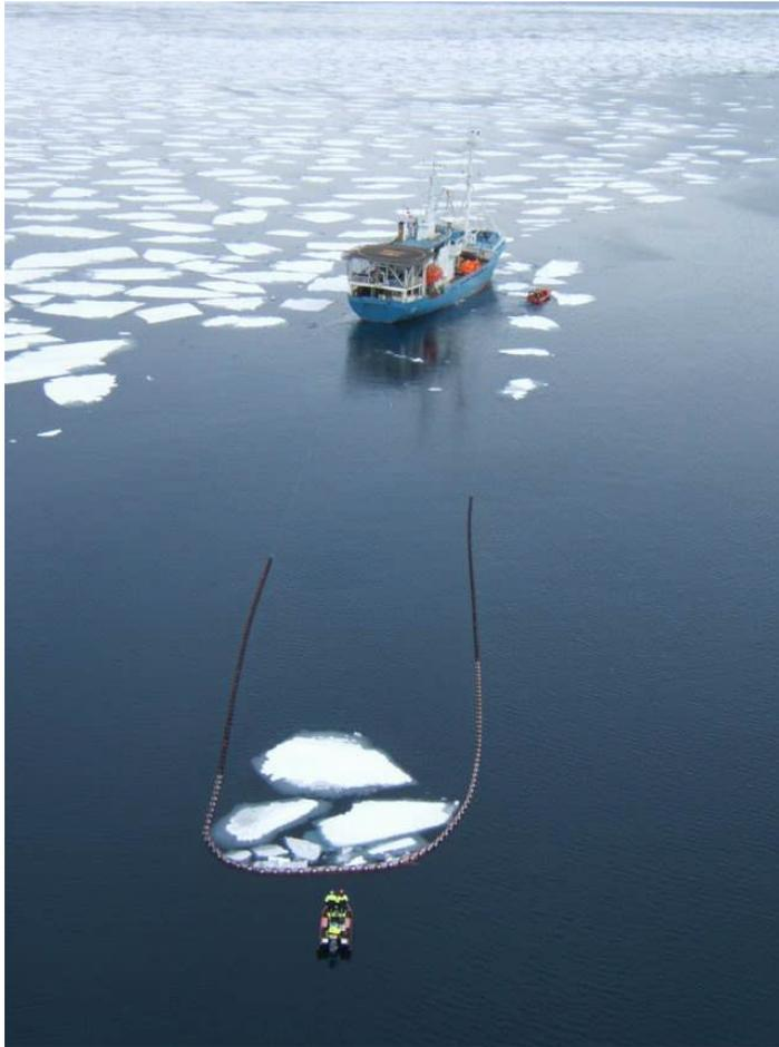
**Figure 4: Applied Fabrics boom under tow with ice**
