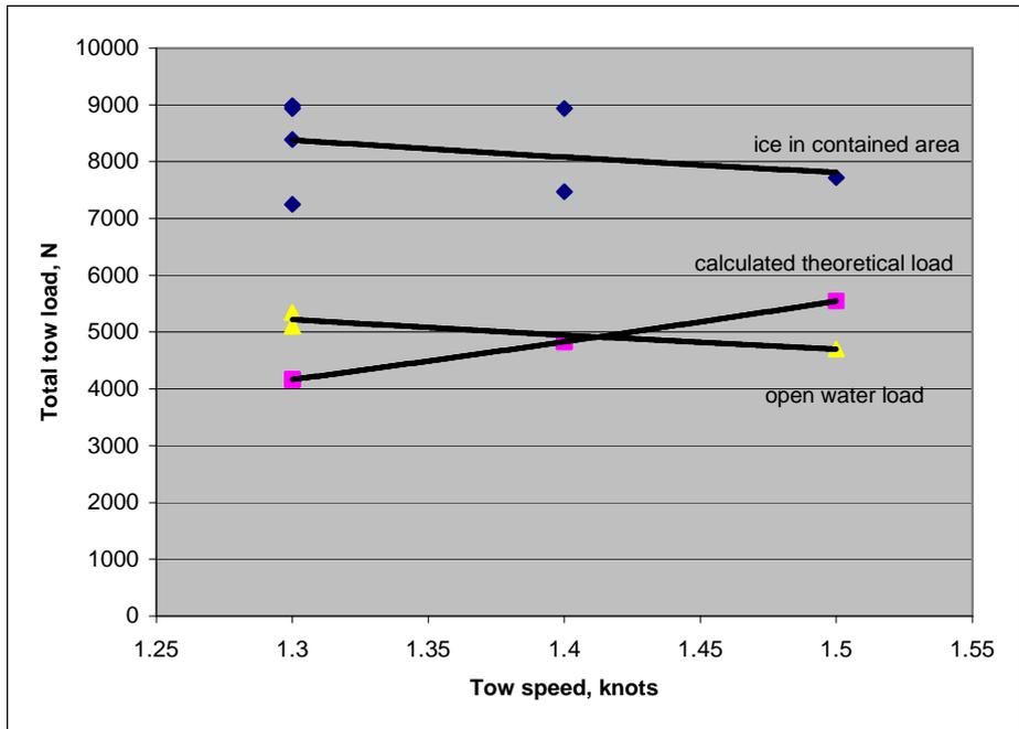
**Figure 7: Tow loads on Elastec boom**
