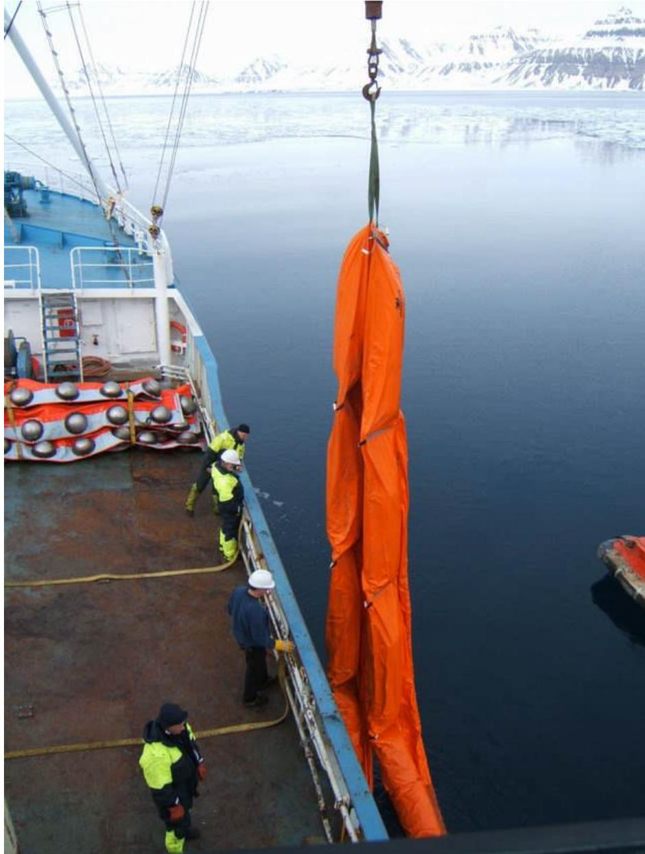
**Figure 1: Retrieving Elastec boom**
