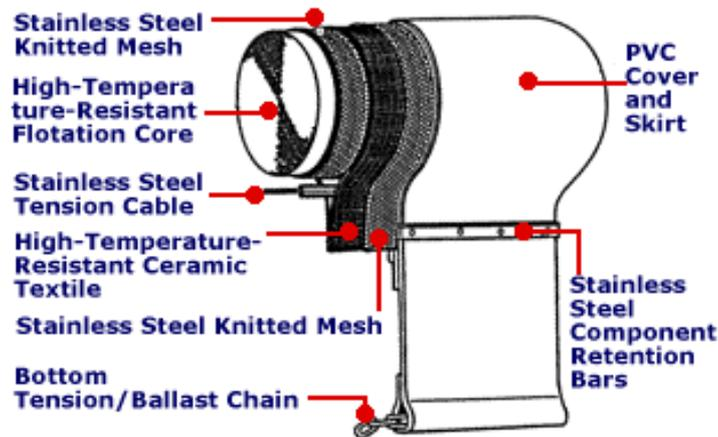
**Figure A-1. Elastec Fireboom Design**
