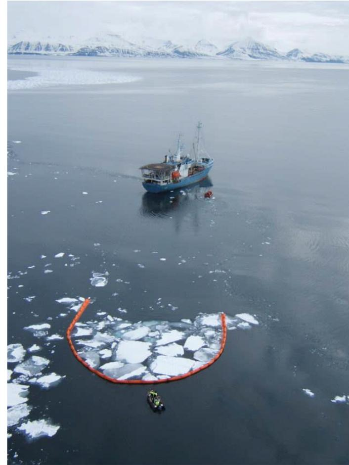
**Figure 5: Elastec boom under tow with ice**
