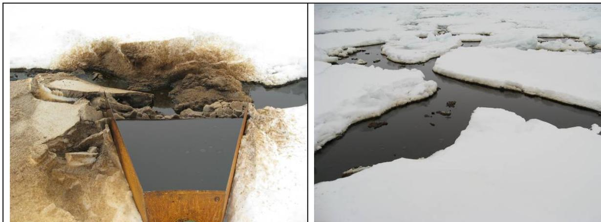
Figure 4.3: Release of 7 m<sup>3</sup> Troll crude oil (Slick P1.2 on May 15<sup>th</sup> 2009). Both RV Lance, the release hose, the overflow chamber and the initial oil slick in the ice is shown in the figure.
