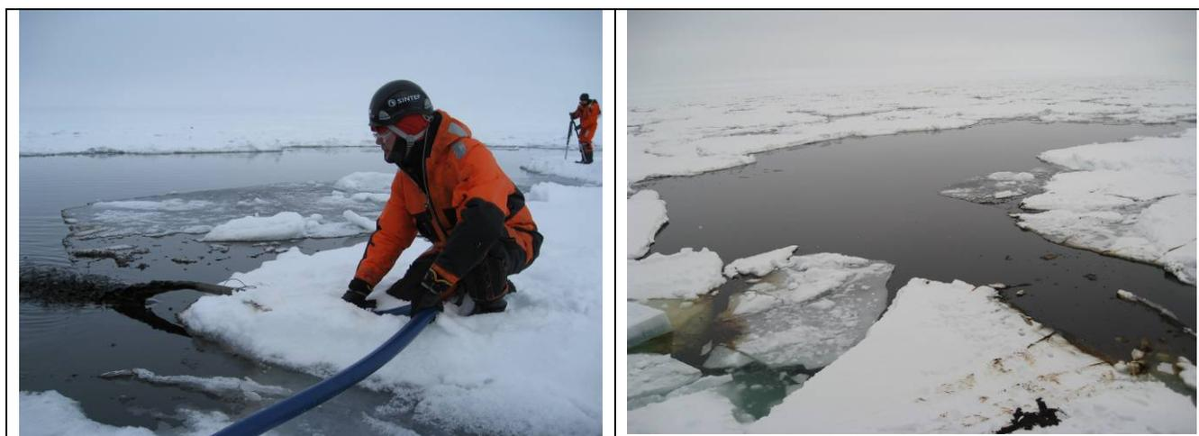
Figure 4.4: Release of 2 m<sup>3</sup> Troll crude oil (Slick P1.1 on May 19<sup>th</sup>). Both the release hose and the initial oil slick in the ice are shown in the figure.
