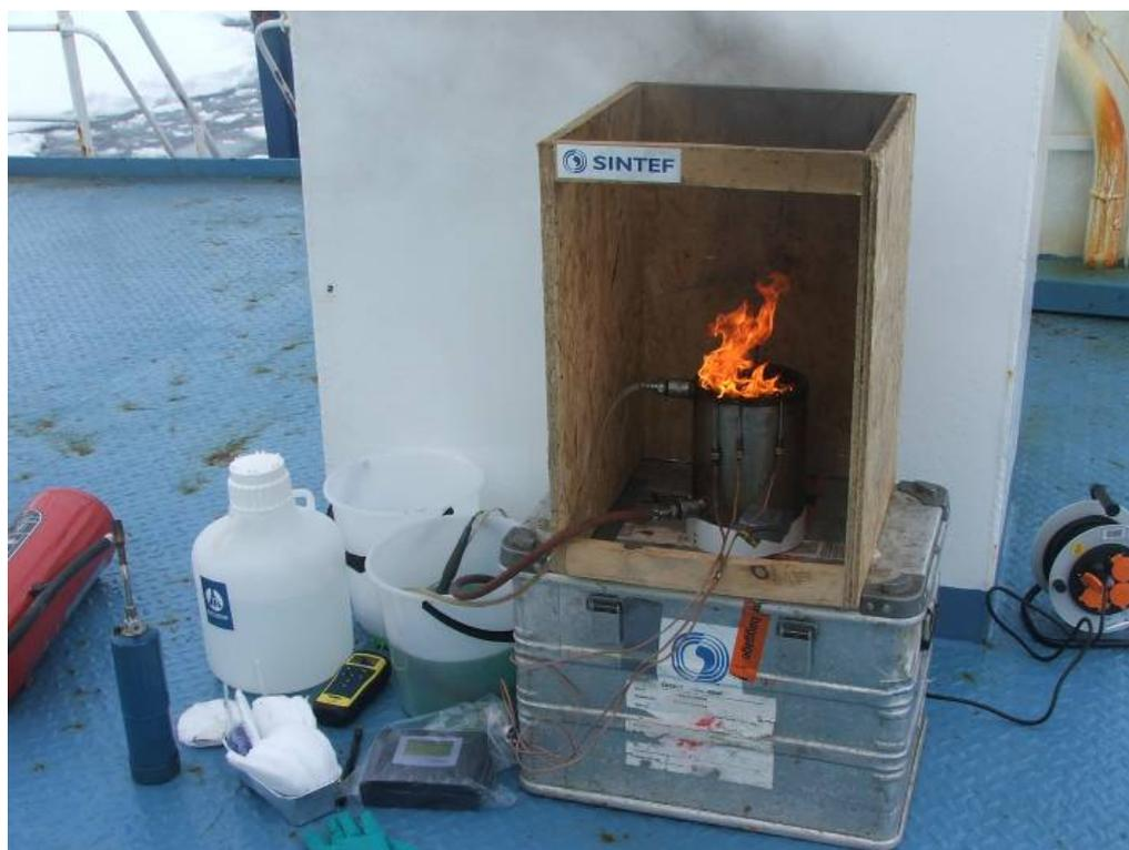
Figure 4.7: Field operation of the burning cell. Cooling system, igniter, thermocouples and the logging unit for flame-, oil- and water temperatures can also be seen.
