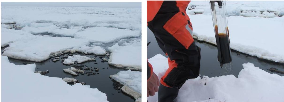
Figure 4.5: The oil immediately after the release (left) and measurement of oil film thickness (right).
