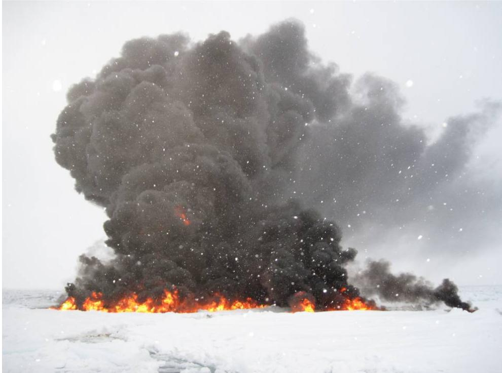
Figure 5.15: In situ burning of 2m<sup>3</sup> weathered free floating Troll B in high ice coverage. The total burn time was 22 minutes. The picture is taken after eleven minutes and is representative for peak intensity.
