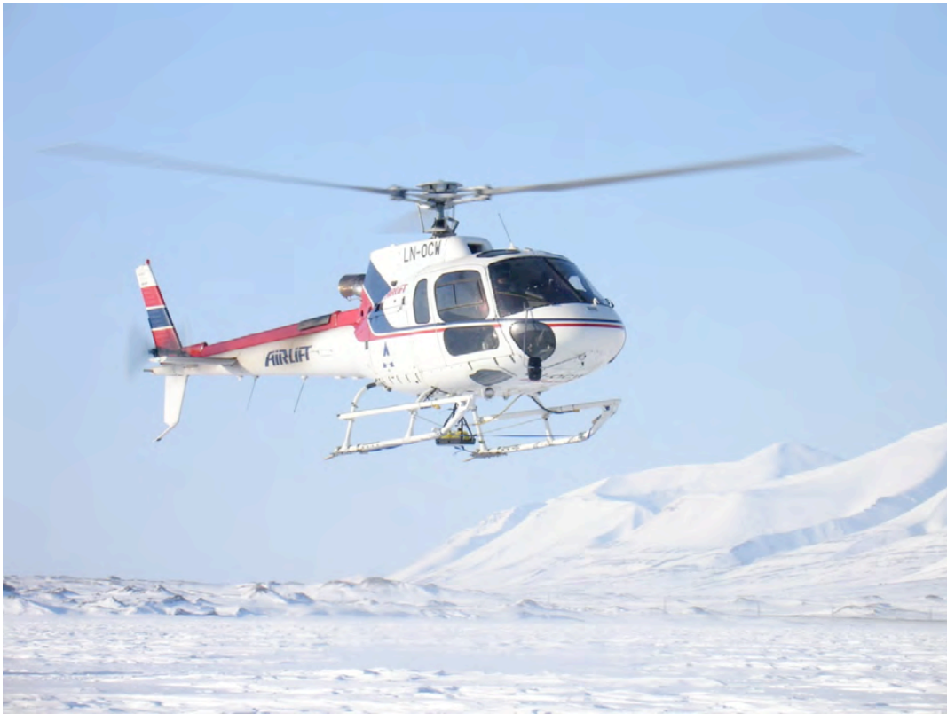
Figure 8. Photograph showing the 1000 MHz shielded antennas suspended from the cargo hook of the helicopter.
