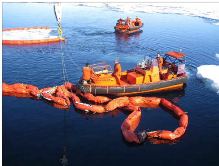
Figure 3.7 Collecting ice in a 25 m boom at the same time as 50 m of boom is installed alongside the vessel. May 14, 2009.
