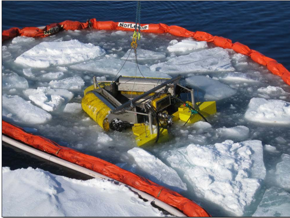
Figure 3.1 Framo skimmer during testing in the field.
