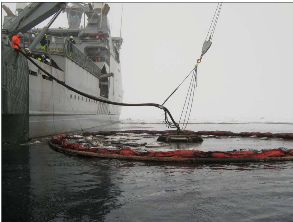
Figure 5.1 Testing of the Polar Bear skimmer during the experimental field trial in May 2009.
