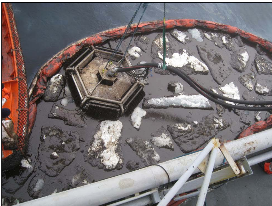
Figure 3.3 Polar Bear skimmer during testing in the field showing hoses supported by ship's crane.
