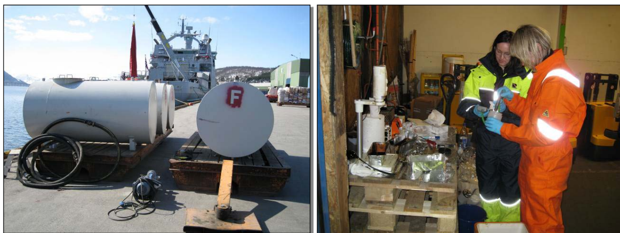
Figure 3.7 Preparation of approximately 8\text{--}9\text{ m}^3 of emulsion along the quay in Tromsø and measurement of water content and viscosity. May 7, 2009.
