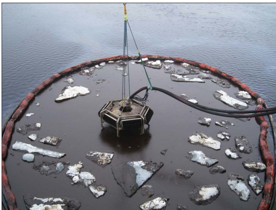
Figure 3.6 Test set-up using a boom of 50 m and an air filled ring to keep the boom in position alongside the starboard side of KV Svalbard. May 16, 2009.
