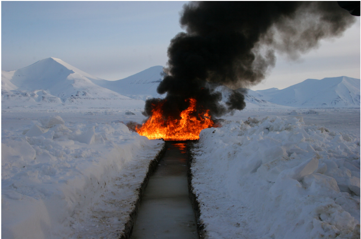
Figure 3.7 In situ burning of weathered oil. The system consisting of a burning basin connected to the weathering basin with a channel (see earlier figure) in operation.
