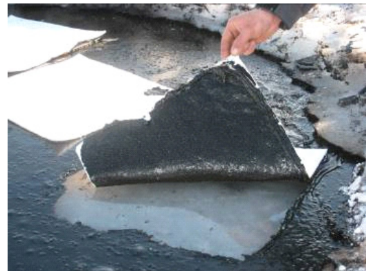
Figure 3.8 Collection of residue. After cooling the residues were easy to remove/collect with 3M adsorption pads. Quantitative collection of residues was important for determining burning effectiveness.
