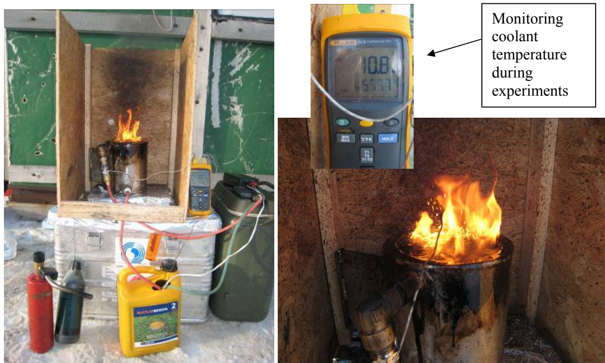
Figure 3.9 The core unit of the laboratory burning cell operated in “Field mode”. Only the cell itself, the butane ignitor, the cooling unit (pump, coolant and thermos), and the flame temperature unit/logger were operated in the field.
