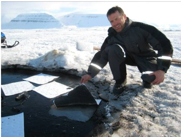
Figure 3.8 Collection of residue. After cooling the residues were easy to remove/collect with 3M adsorption pads. Quantitative collection of residues was important for determining burning effectiveness.
