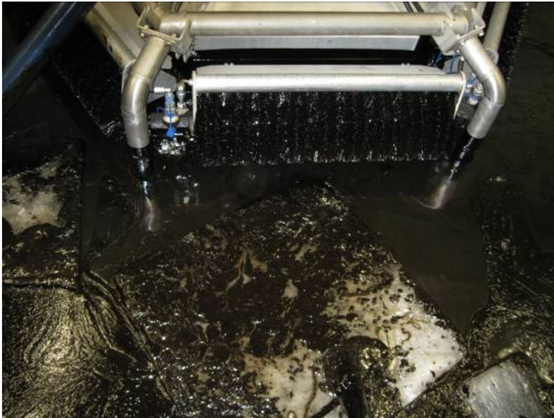
Figure 4.1 Flow of emulsion towards the skimmer is limited by ice
