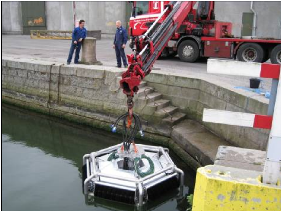
Figure 1.2 Testing of floating characteristics in Ålborg harbour.
