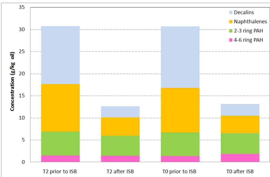
Figure 3.11 Oil composition (in g analyte/kg oil) prior to and after ISB. T0 was ignited within one hr after oil release and T2 after two days. A VOC analysis was not performed.
