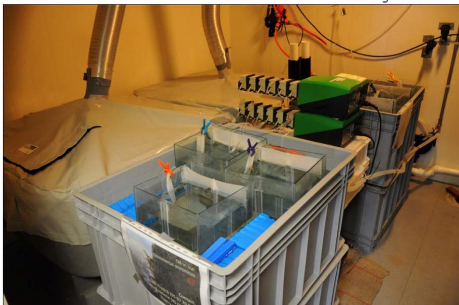
*Figure 2.3 General view of experimental setup. Each header-tank fed three exposure aquaria.*
