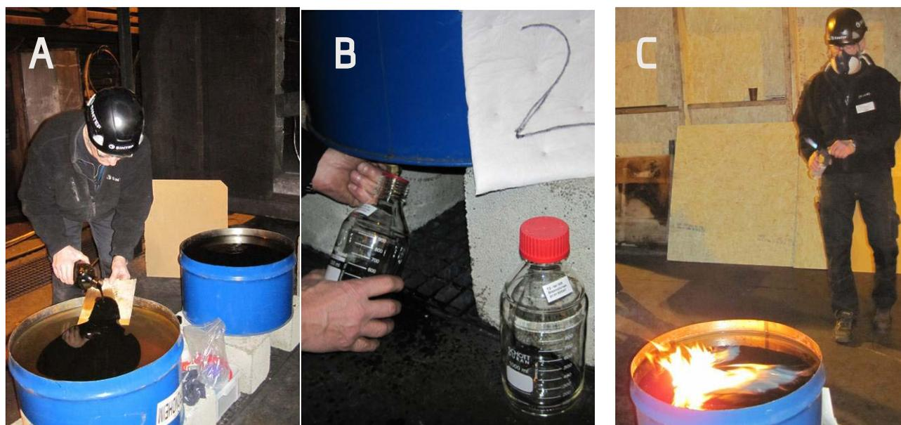
Figure 2.4 Oil application (A), water sampling (B), and ignition (C).
