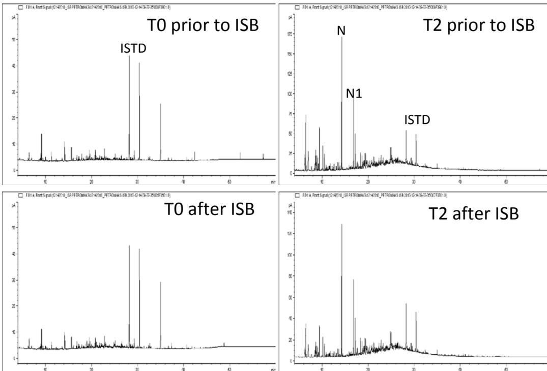
Figure 3.9 GC chromatograms of water prior to and after ISB. The peaks for the added internal standards (ISTD, two peaks) and naphthalene (N) and C1-naphthalenes (N1) are labelled.
