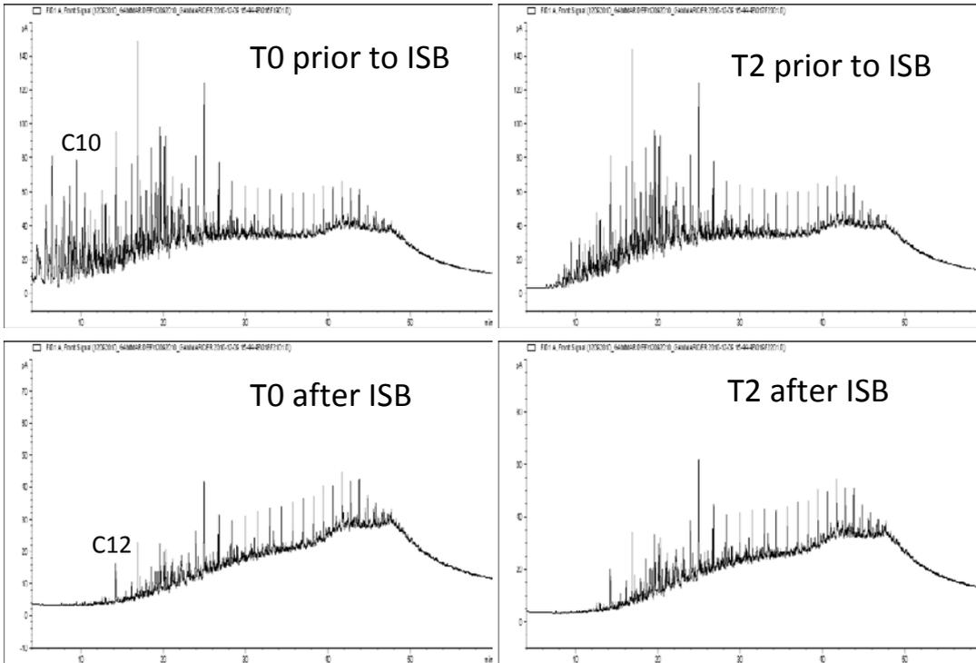
Figure 3.8 GC chromatograms of the oil slick prior to and after ISB. T0 was ignited within one hr after the oil release and T2 after two days.
