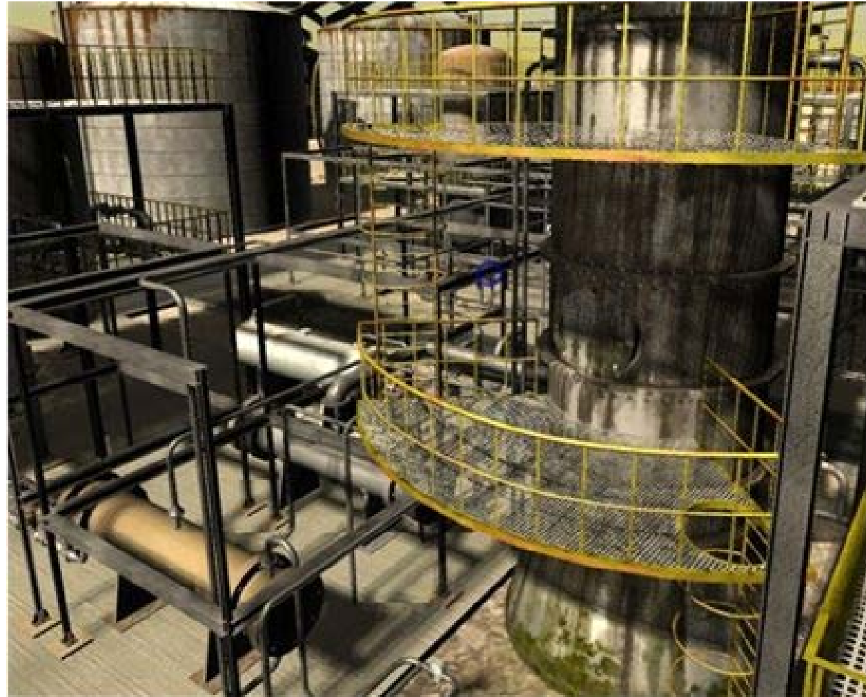
3D representation of a distillation column (vertical cylinder on the right), and of auxiliary process units such as reboiler, condenser, and reflux drum (i.e. the three horizontal cylinders from left-bottom corner to the center of the figure)
