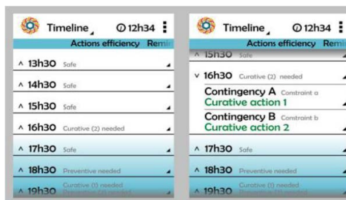
Figure 24: GUI proposed in iTesla for risk visualization in the short-term 4
