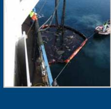
Floating elements for correct positioning of the skimmerboom
