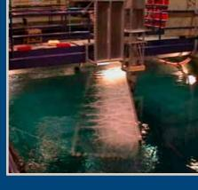
• Study and quantify the structure of a near-surface, area bubble source and how the surface outwelling flow varies with the number of spargers and air flow rate.
