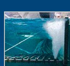
A downstream skirt extending from the surface to the bubble source depth of 60 cm was used to simulate a combined bubble oil boom (BOB) (Fig 4 - Fig 6). • The tests mapped the velocity structure in far greater
