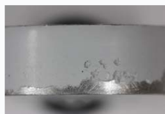
Erosion pattern observed on a PU-coating doped with 5 wt% N2 at 140 m/s for 60 min.
