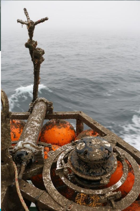
Substantial biofouling after 4 month deployment at FINO1
