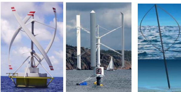
Figur 1 Examples of VAWTs: a) Gwind [1] b) Seatwirl [2] c) Deepwind [3]
