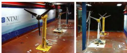
Figure 2: Tandem Setup in the wind tunnel.
