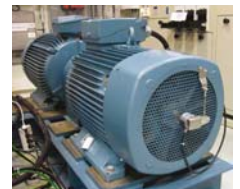
55 kW wind turbine emulator. Fixed speed induction generator.
