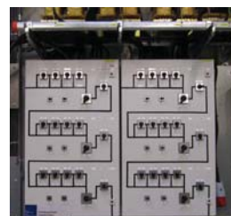
Distribution line model, RLC line section equivalents.
