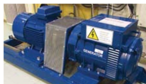
17 kW hydropower generator model. Control equipment typically found in 1-10 MW power plants.
