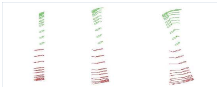
Figure 5: Two NACA 0012 wings rotating. The pitch angle is constant, and the illustration is showing the wake development at three different stages in time.
