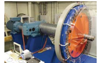
50 kW low speed (30rpm) Permanent Magnet Synchronous generator
