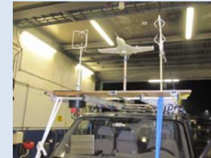
Fig 5: Setup for the test campaign at Flesland airport. From left to right: Gill R3-100 sonic anemometer, SUMO dummy with the 5-hole turbulence probe, Campbell CSAT3 sonic anemometer.
