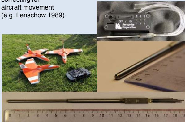
Fig 1: The SUMO system and the 5-hole probe turbulence sensor.
