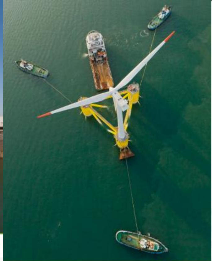
Aguçadoura WindFloat Prototype October 2011 - Sado River near Setubal, Portugal
