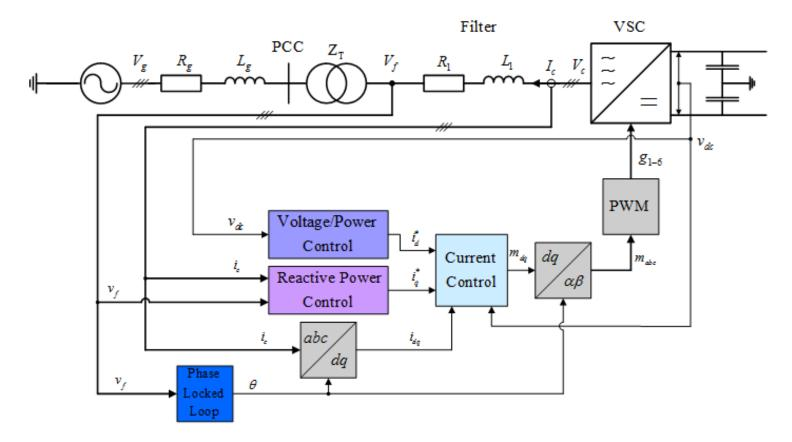
Synchronized to onshore power system by Phase Locked Loop (PLL)
