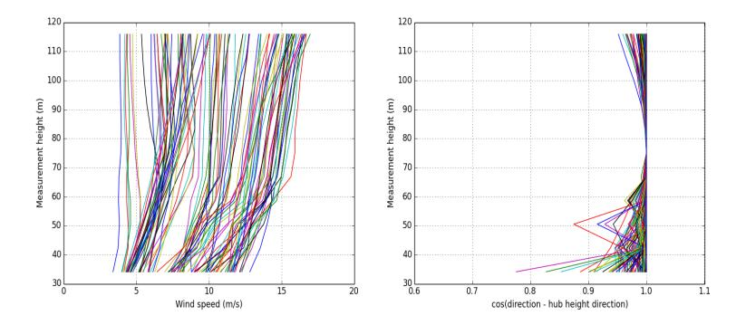
**Vertical wind shear and TI**. Both these quantities are influenced by atmospheric stability, and can have a significant effect on turbine performance. This is reflected in power curve measurements. Unless account of these effects is included, power curves will have larger uncertainties
