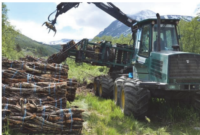
Figure 9: John Deere bundler in action. (photo: Leif Kjøstelsen)
