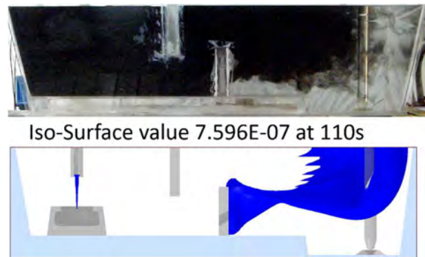
Figure 9: Black ink dispersion photo in the water model compared to tracer concentration iso-surface of mathematical model at time 110s.
