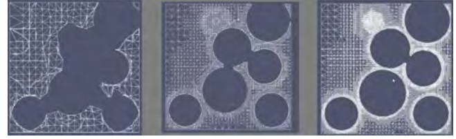
Figure 3: Grain surface definition at three increasing mesh refinement levels.
