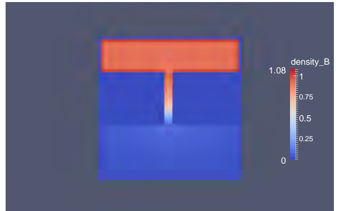
Figure 6: Meniscus in a rectangular pore throat which is 3 LB units wide.
