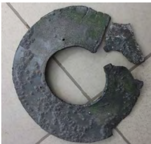
Figure 17: The metal plate found in a the bottom of Secondary Reformer (Pilbara)
