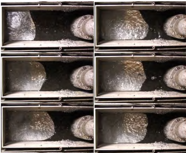
Figure 11: Video snapshots of the metal slag interface during argon injection tests at CCS-1 (taken every 10 seconds for a total time of 1 minute) for an argon mass flow rate=4 lt/min.
