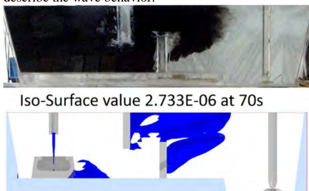
Figure 8: Black ink dispersion photo in the water model compared to tracer concentration iso-surface of mathematical model at time 70s.
