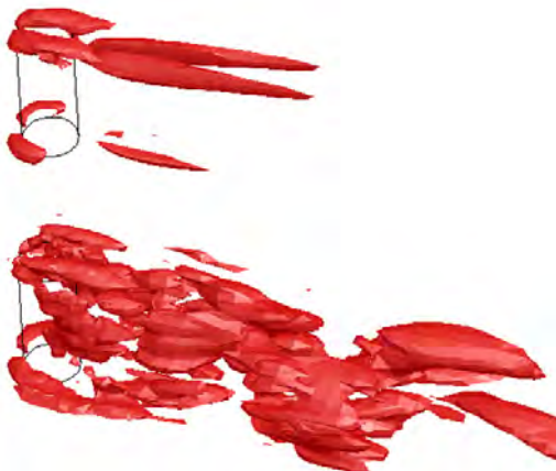
Figure 4: Iso-surface of helicity magnitude, H = |\mathbf{u} \cdot (\nabla \times \mathbf{u})| as result of conventional finite volume based URANS simulation (top) and embedded LB simulations (bottom); in the latter case unsteady vortex shedding is observed.
