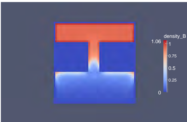
Figure 5: Meniscus in a rectangular pore throat which is 5 LB units wide.
