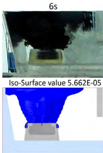
Figure 7: Black ink dispersion photo in the water model compared to simulated tracer concentration iso-surface of mathematical model at time 6s.
