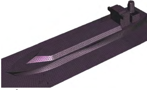
Figure 2. The mesh: the simplified model of the membrane ship.
