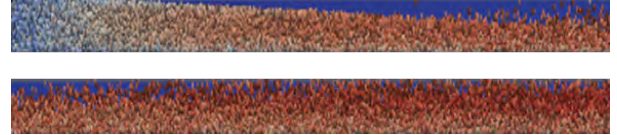
Figure 4: Particle dispersion in the channel showing re-suspension after a tendency for settling (two parts of the channel).
