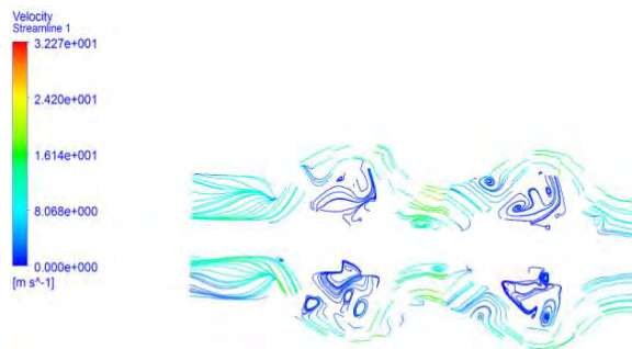
Figure 13. Streamlines on the section AA, case 3, liquid phase
