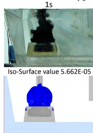
Figure 6: Black ink dispersion photo in the water model compared to simulated tracer concentration iso-surface of mathematical model at time 1s.
