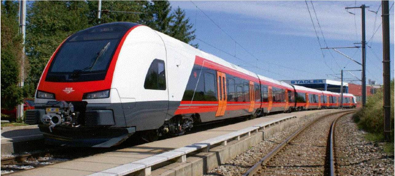
Figure 7-4-part electrical train of the FLIRT family
