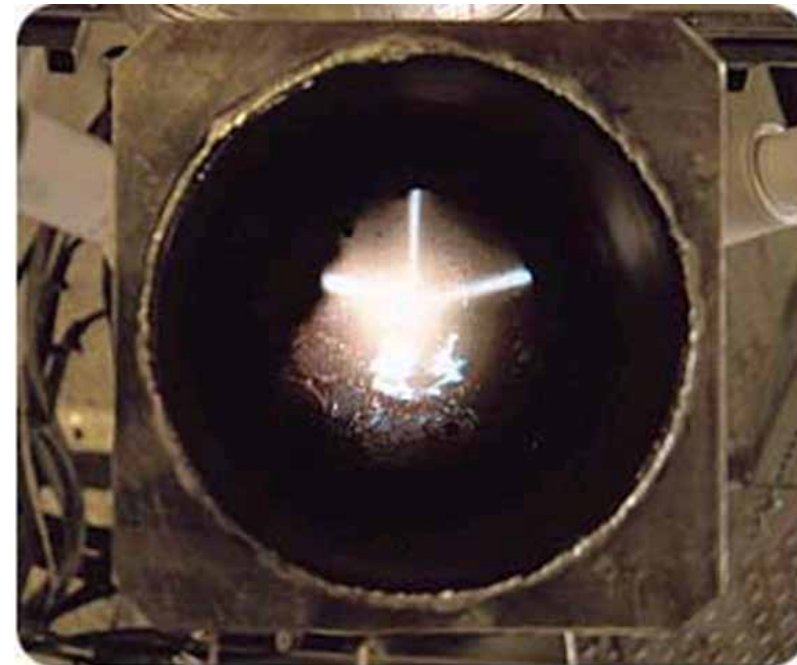
Three Transferred Plasma arcs in the Plasma REactor for Smelting at SINTEF (PRESS)
