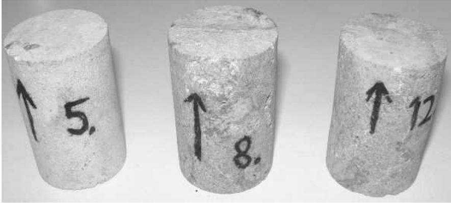
**Fig. 2.5.** Three core plugs with diameter of one and a half inches, and a height of five centimetres.
