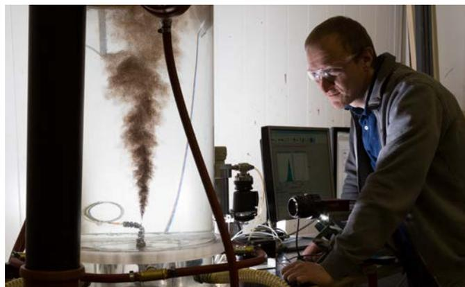
*SINTEF MiniTower can be used as a bench-scale test for subsea dispersant effectiveness*
