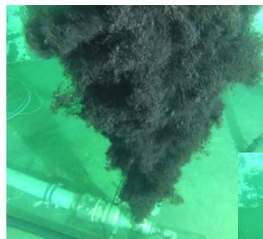
TowerBasin experiment with the 32 mm nozzle and 120 L/min of Oseberg blend (left)
