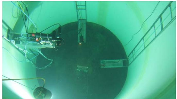
All three instrument platforms lowered and ready to initiate an experiment. The squared release platform can be seen in the middle on the bottom of the tank.
