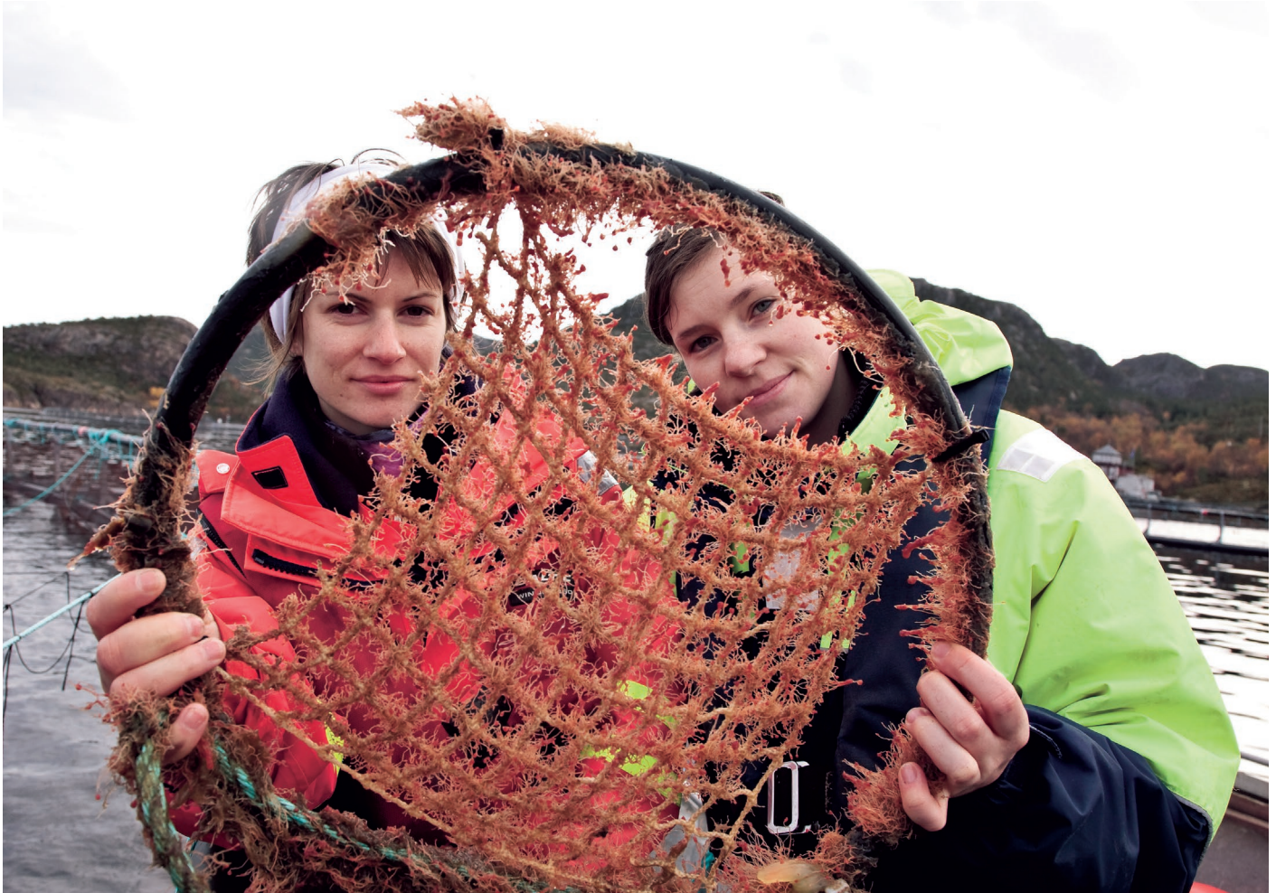
Scientists are trying to find ways to both prevent and remove net fouling, one of the main challenges facing aquaculture today. Nets can quickly become blocked, preventing water-flow through the sea-cage and thus the essential supply of oxygen for the fish. Photo: SINTEF/Thor Nielsen
