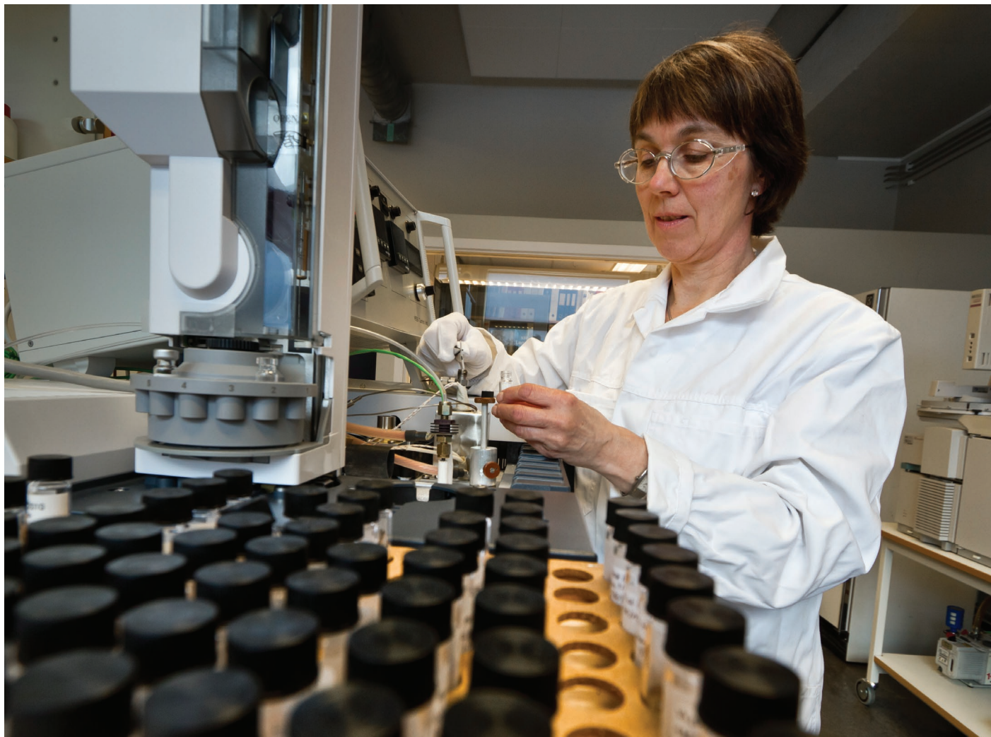
Kristin Lind in the organic geochemistry laboratory. Here she is analysing hydrocarbons in a sample of source rock by means of Micro-Scale Sealed Vessel (MSSV) pyrolysis. Photo: SINTEF/Thor Nielsen
