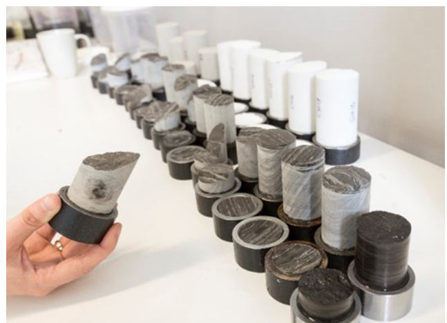
Samples from shale and chalk tested for tensile strength.
