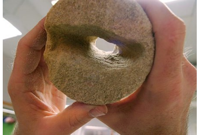
Post-test photograph of sandstone hollow cylinder sample
